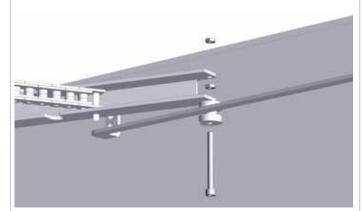
Mount the wheel under the motor arm using the supplied bolt. Make sure that the wheel is mounted behind the bracket **WDB 820M**. Fasten the nuts with a torque of 2 Nm.
