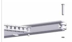
Remove the lockwasher and the pin.
