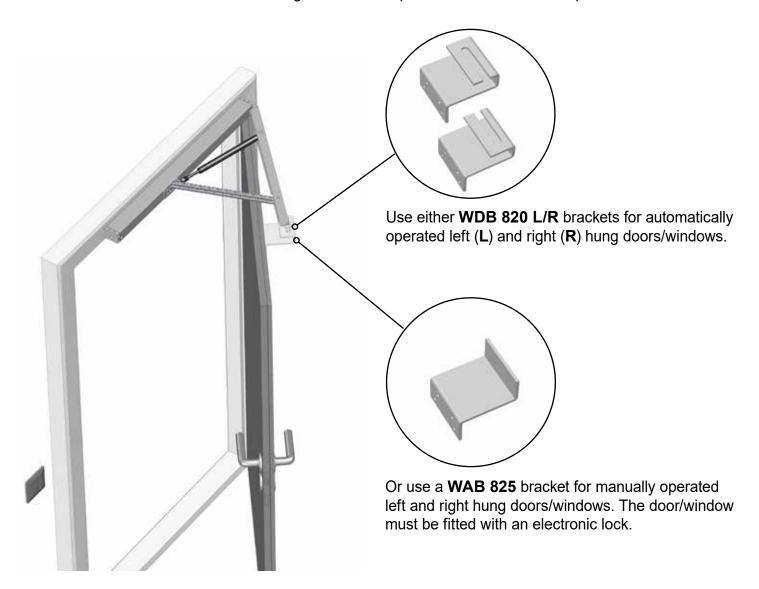
**Manually operated door**Left hung inward opening door in an aluminium frame. The door can be manually operated and must be fitted with an electronic lock.
