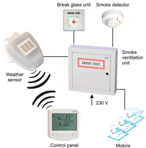
10.5.b In connection with Smoke ventilation unit WSC
